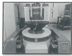
Battery Condition: Fully charged (100% SOC), contained at ambient temperature, firmly held on the vibration table in vehicle mounting position. Vibration test will be carried out in three-axis viz. in the vertical axis, horizontal axis and battery positioned in longitudinal direction. Acceleration: 3 g (sinusoidal vibration)
